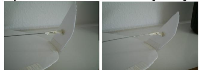
Fig. 20. The deflection of the winglet on the MAV. Note the mechanical linkage.
