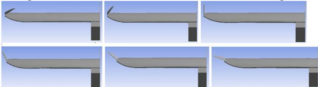
Fig. 4. CAD model of different winglet angle, from the top left to bottom right are:-50,-30,0,20,45,65 degree.
