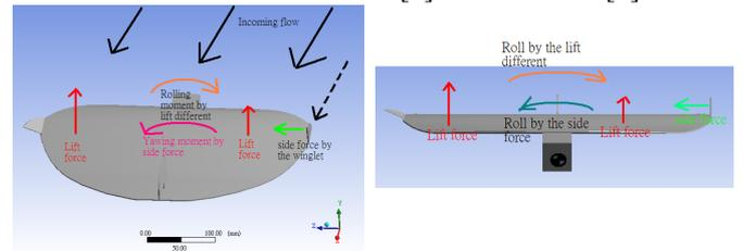
Fig. 19. Asymmertic winglet MAV during the turn. (front view at right)
