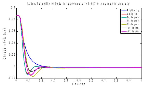
Fig. 11. Lateral stability results of the MAV (change in  $\beta$ )
