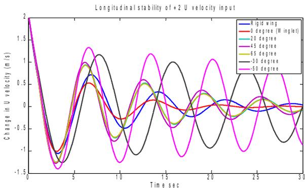
Fig. 9. Longitudinal stability results of the MAV (change in U velocity)
