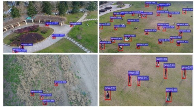
Figure 7: Human detection results using our WiSAR system.
