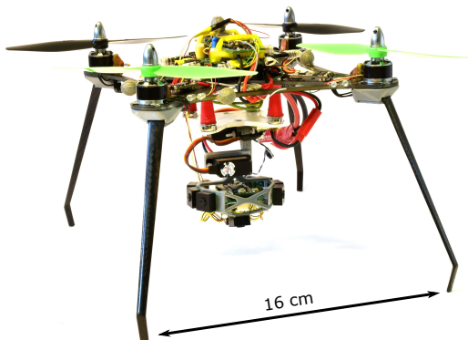
Figure 1: Photograph of the X4-MaG quadrotor with the gimbal case attached below (total mass: 395 g, span: 30 cm, autonomy: 6 min).
