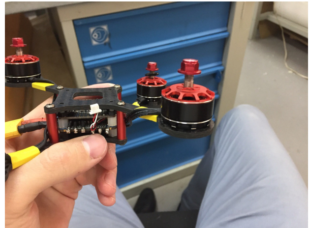
Figure 3: Double deck frame
