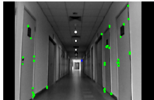
Figure 11: Detected features in long corridor.
