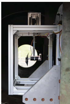
(a) ISAE-SUPAERO's experimental testbed in the depressurised tank
