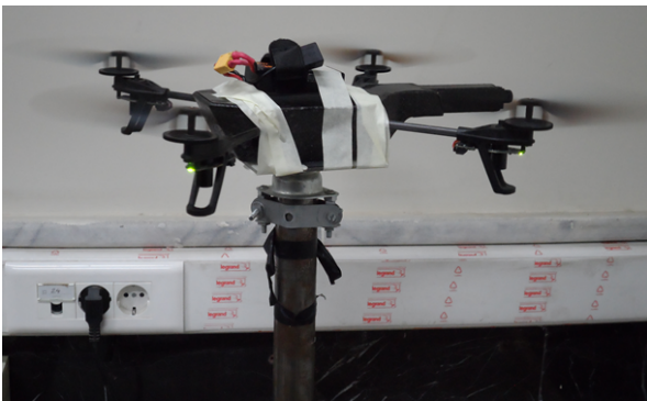
Figure 2: Experimental test bed of a 3-DOF quadrotor in the AUTMAV laboratory.
