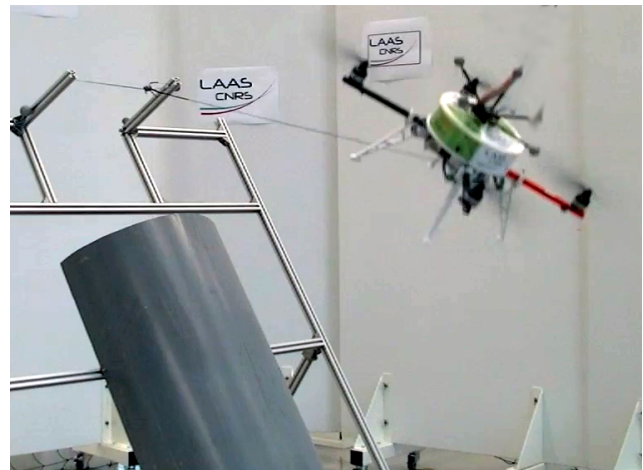
Figure 1: Tethered landing on a sloped pipe tilted by 60^\circ .
