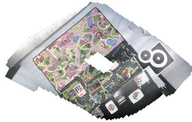
Figure 3: The created map (size: approximately 5 \times 5 meters) that was stitched together using 800 images.
