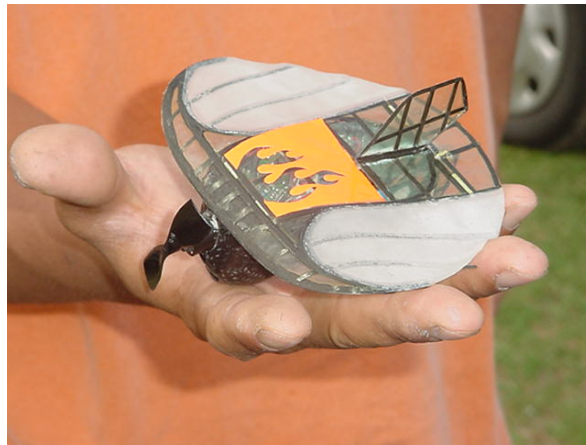
Figure 3: MAV propeller with cut blades
