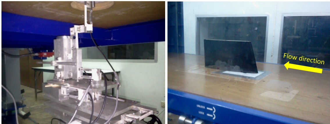
Figure 4: 3-component balance with turn table and model setup
